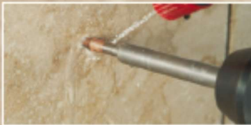
PTC Carbide shown with water cooling system, quickly producing a hole in porcelain tile
